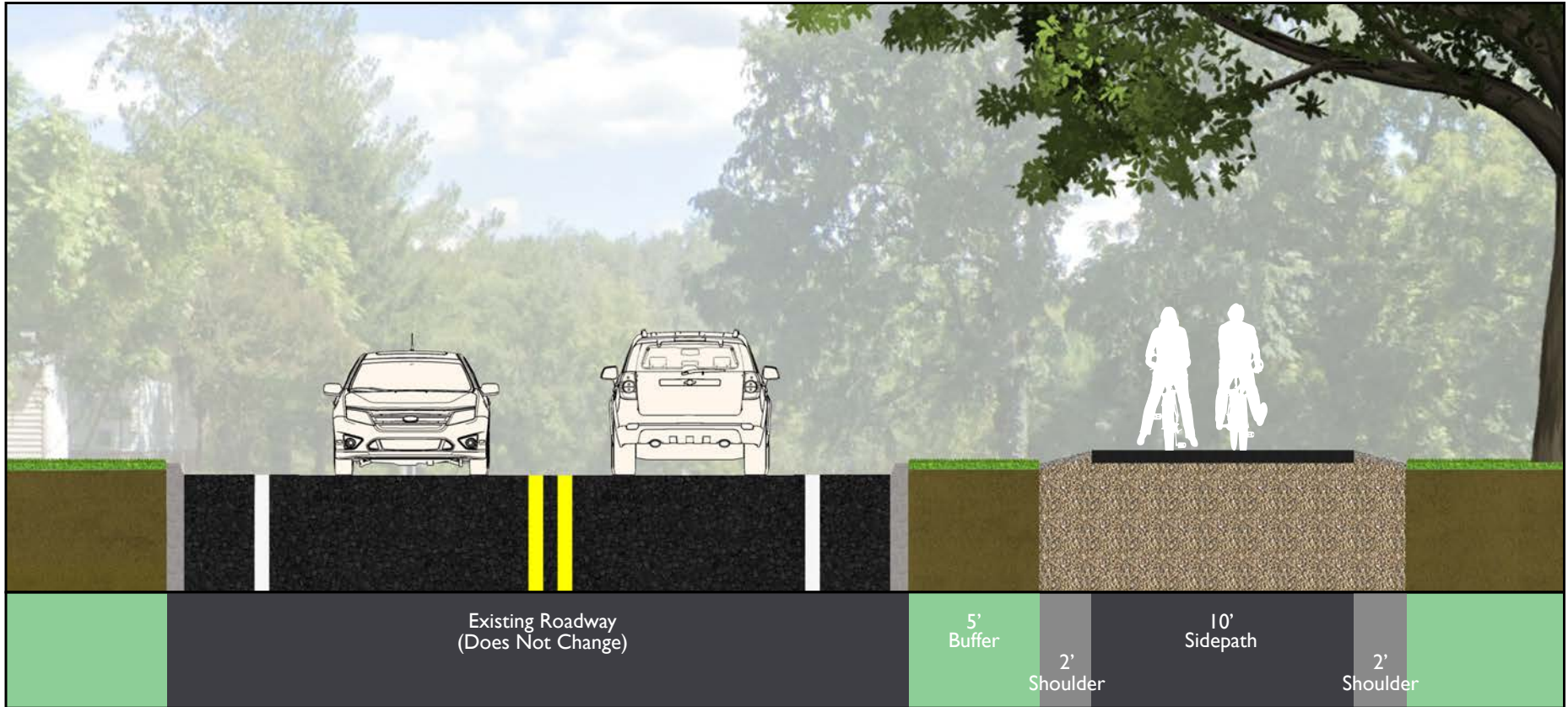
Image 58. 10-Foot Sidepath (12-Foot Where Feasible) Typical Cross Section on 4th Avenue East
